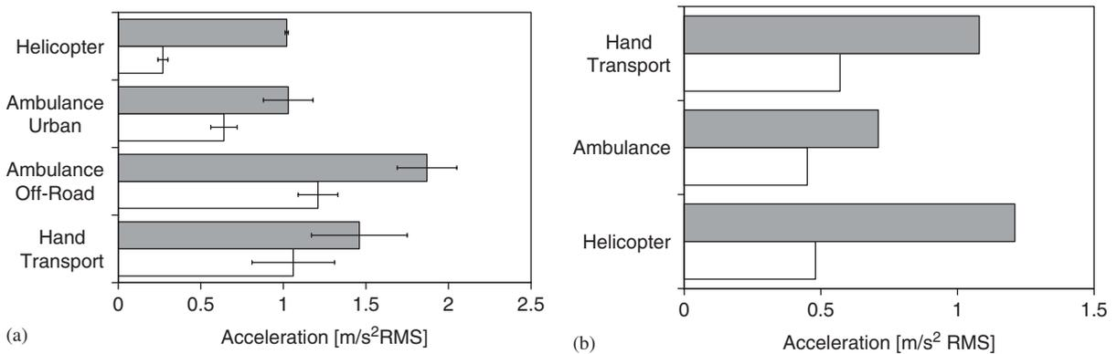
Fig. 7. Comparison of vibration total values at the stretcher–injured interface with different means of transportation (a) and in different load–unload operations (b).
