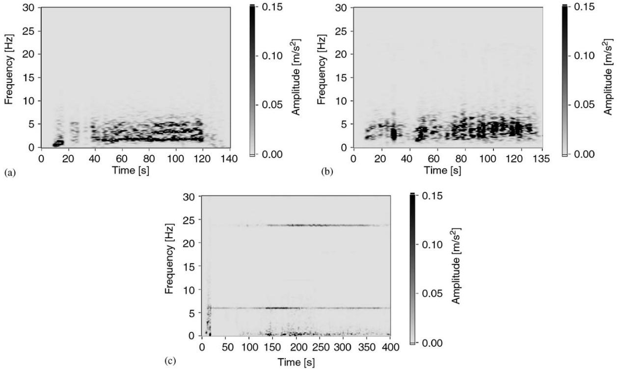
Fig. 4. Short time Fourier transform of the seat-pad X accelerations in different transport conditions: (a) hand transport, skilled operators, (b) ambulance transport on off-road terrain, and (c) helicopter: stretcher-loading and cruise. X-axis time [s], Y-axis frequency [Hz], Color scale acceleration values [m/s<sup>2</sup> rms].
