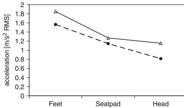
Fig. 6. Acceleration measured on the stretcher at feet, center of gravity and head position. Head is toward the front of the vehicle. — Δ— unweighted acceleration values, —●— Weighted acceleration values.
