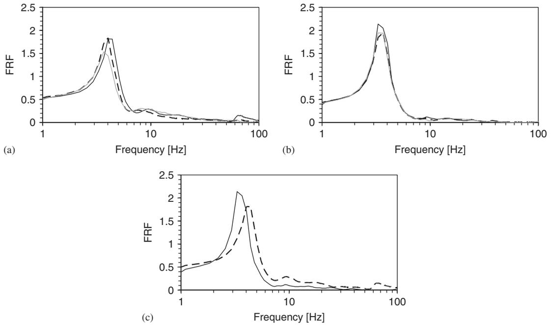
Fig. 3. Changes in FRF due to: (a) patient’s body mass (— 70 kg, ---- 80 kg, —·— 90 kg); (b) nonlinearities (— 4.5 m/s<sup>2</sup>, ---- 5.4 m/s<sup>2</sup>, —·— 6.3 m/s<sup>2</sup>); (c) use of shafts (— with shafts, ---- without shafts).
