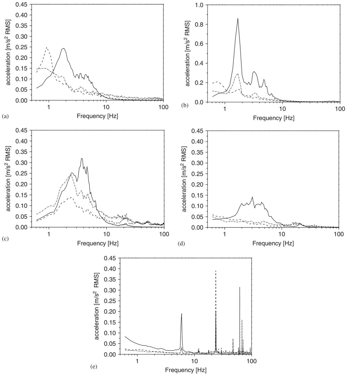
Fig. 5. Acceleration spectra at the injured–stretcher interface in different conditions: (a) hand transport, skilled operators, (b) hand transport, novices, (c) ambulance, off-road, (d) ambulance, urban, and (e) helicopter loading and cruise; — seat-pad *X*-axis, - - - seat-pad *Y*-axis, ···· seat-pad *Z*-axis.
