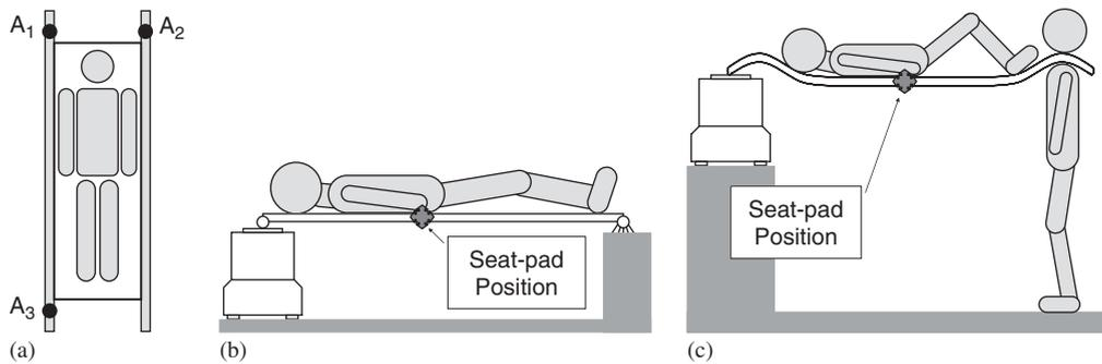
Fig. 2. Accelerometers position (a) and experimental setup (b, c) for stretcher dynamic characterization.
